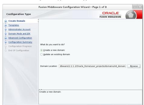
Run the config.sh from <ORACLE\_HOME>/oracle\_common/common/bin folder. The Configuration Type window appears.
